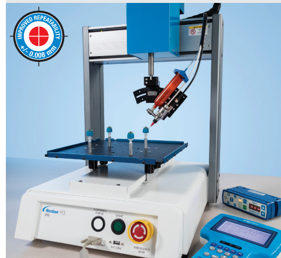
R Series makes 4-axis dispensing automation easy.
